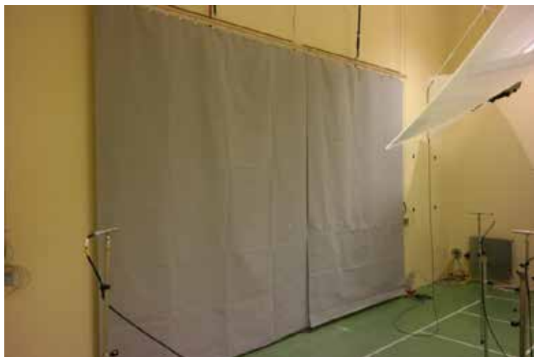
Picture 1: Test item Polaris with flat-arrangement in the reverberation room
